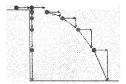
If the time it takes for the marble to reach  $\Delta x_x$  (range in the x direction) is the same as the amount of time it takes for a marble in free-fall from the same height ( $\Delta x_y$ ), one can find the time the projectile will be in flight given the distance.
